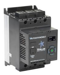
Stellar SR35 series basic soft starter, 27A, 110-240 VAC at 1-phase/208-460 VAC at 3-phase, Trip Class 10/20/30, rated for 5 start/hour, internally bypassed, 1 frame.
