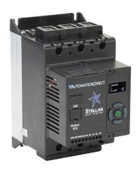
Stellar SR35 series basic soft starter, 22A, 110-240 VAC at 1-phase/208-460 VAC at 3-phase, Trip Class 10/20/30, rated for 5 start/hour, internally bypassed.
