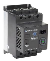
Stellar SR35 series basic soft starter, 17A, 110-240 VAC at 1-phase/208-460 VAC at 3-phase, Trip Class 10/20/30, rated for 5 start/hour, internally bypassed.
