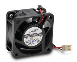
Stellar SR22 series main cooling fan,  $40 \times 40 \times 20$ mm, 24 VDC, increases duty cycle to 60 starts/hour. For use with SR22-22, SR22-30, SR22-36 and SR22-40 soft starters.
