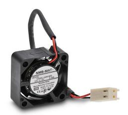
Stellar SR22 series main cooling fan,  $25 \times 25 \times 10$ mm, 12 VDC, increases duty cycle to 60 starts/hour. For use with SR22-05, SR22-07, SR22-09, SR22-12 and SR22-16 soft starters.
