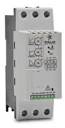
Stellar SR22 series compact soft starter, 36A, 110-240 VAC at 1-phase/208-460 VAC at 3-phase, Trip Class 2/10/20, rated for 10 start/hour, internally bypassed.
