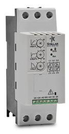
Stellar SR22 series compact soft starter, 36A, 110-240 VAC at 1-phase/208-460 VAC at 3-phase, Trip Class 2/10/20, rated for 10 start/hour, internally bypassed, 55mm frame.
