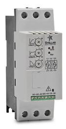
Stellar SR22 series compact soft starter, 30A, 110-240 VAC at 1-phase/208-460 VAC at 3-phase, Trip Class 2/30, rated for 10 start/hour, internally bypassed, 55mm frame.
