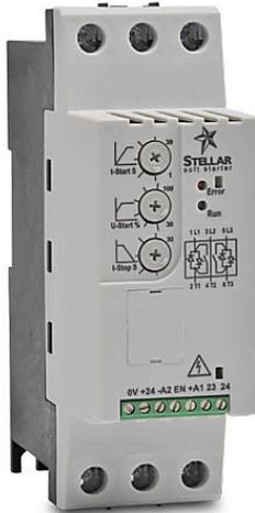
Stellar SR22 series compact soft starter, 30A, 110-240 VAC at 1-phase/208-460 VAC at 3-phase, Trip Class 2/30, rated for 10 start/hour, internally bypassed, 55mm frame.
