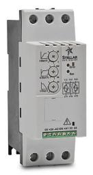
Stellar SR22 series compact soft starter, 22A, 110-240 VAC at 1-phase/208-460 VAC at 3-phase, Trip Class 2/10/20/30, rated for 10 start/hour, internally bypassed.
