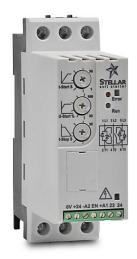
Stellar SR22 series compact soft starter, 16A, 110-240 VAC at 1-phase/208-460 VAC at 3-phase, Trip Class 2/10/20/30, rated for 10 start/hour, internally bypassed, 45mm frame.
