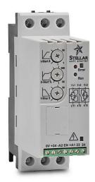
Stellar SR22 series compact soft starter, 12A, 110-240 VAC at 1-phase/208-460 VAC at 3-phase, Trip Class 2/10/20/30, rated for 10 start/hour, internally bypassed.
