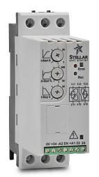
Stellar SR22 series compact soft starter, 9A, 110-240 VAC at 1-phase/208-460 VAC at 3-phase, Trip Class 2/10/20/30, rated for 10 start/hour, internally bypassed, 45mm frame.
