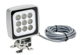
CCEA SIRIO Q series LED work light, 100 x 100 x 25mm, 12-24 VDC operating voltage, daylight white, 5000K, 16W, 1450 lm, bracket mount, pigtail, aluminum body, 9.8ft/3m cable length, IP67 and IP69. Mounting bracket included.
