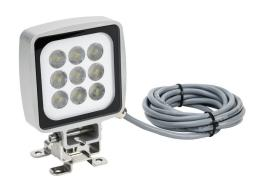
CCEA SIRIO Q series LED work light, 100 x 100 x 25mm, 12-24 VDC operating voltage, daylight white, 5000K, 16W, 1450 lm, bracket mount, pigtail, aluminum body, 9.8ft/3m cable length, IP67 and IP69. Mounting bracket included.
