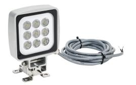
CCEA SIRIO Q series LED work light, 100 x 100 x 25mm, 12-24 VDC operating voltage, daylight white, 5000K, 16W, 1750 lm, bracket mount, pigtail, aluminum body, 9.8ft/3m cable length, IP67 and IP69. Mounting bracket included.
