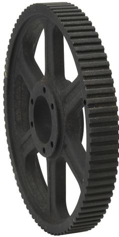
SureMotion timing pulley, cast iron, 3/8in L pitch, 84 tooth, 10.027in pitch diameter, no hub without flanges. For use with 1in wide belt. Requires SD series QD style bushing.
