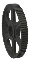
SureMotion timing pulley, cast iron, 3/8in L pitch, 84 tooth, 10.027in pitch diameter, no hub without flanges. For use with 1in wide belt. Requires SD series QD style bushing.
