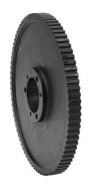
SureMotion timing pulley, cast iron, 3/8in L pitch, 84 tooth, 10.027in pitch diameter, no hub without flanges. For use with 1/2in wide belt. Requires SD series QD style bushing.
