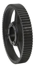
SureMotion timing pulley, cast iron, 3/8in L pitch, 72 tooth, 8.594in pitch diameter, no hub without flanges. For use with 1in wide belt. Requires SD series QD style bushing.
