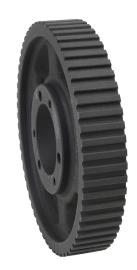
SureMotion timing pulley, cast iron, 3/8in L pitch, 60 tooth, 7.162in pitch diameter, no hub without flanges. For use with 1in wide belt. Requires SD series QD style bushing.
