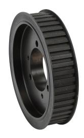
SureMotion timing pulley, ductile iron, 3/8in L pitch, 48 tooth, 5.73in pitch diameter, no hub with flanges. For use with 1in wide belt. Requires SDS series QD style bushing.
