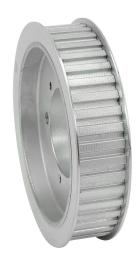
SureMotion timing pulley, ductile iron, 3/8in L pitch, 44 tooth, 5.252in pitch diameter, no hub with flanges. For use with 1in wide belt. Requires SDS series QD style bushing.
