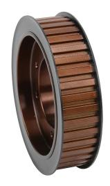
SureMotion timing pulley, ductile iron, 3/8in L pitch, 40 tooth, 4.775in pitch diameter, no hub with flanges. For use with 1in wide belt. Requires SDS series QD style bushing.
