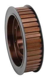
SureMotion timing pulley, ductile iron, 3/8in L pitch, 40 tooth, 4.775in pitch diameter, no hub with flanges. For use with 1in wide belt. Requires SDS series QD style bushing.
