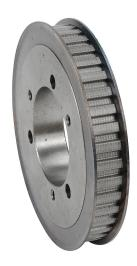
SureMotion timing pulley, ductile iron, 3/8in L pitch, 40 tooth, 4.775in pitch diameter, no hub with flanges. For use with 1/2in wide belt. Requires SDS series QD style bushing.
