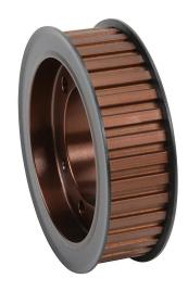
SureMotion timing pulley, ductile iron, 3/8in L pitch, 36 tooth, 4.297in pitch diameter, no hub with flanges. For use with 1in wide belt. Requires SDS series QD style bushing.
