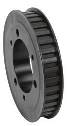
SureMotion timing pulley, ductile iron, 3/8in L pitch, 36 tooth, 4.297in pitch diameter, no hub with flanges. For use with 1/2in wide belt. Requires SDS series QD style bushing.
