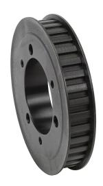
SureMotion timing pulley, ductile iron, 3/8in L pitch, 36 tooth, 4.297in pitch diameter, no hub with flanges. For use with 1/2in wide belt. Requires SDS series QD style bushing.
