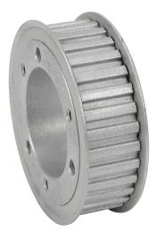
SureMotion timing pulley, ductile iron, 3/8in L pitch, 32 tooth, 3.82in pitch diameter, no hub with flanges. For use with 1in wide belt. Requires SDS series QD style bushing.
