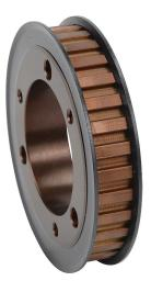
SureMotion timing pulley, ductile iron, 3/8in L pitch, 32 tooth, 3.82in pitch diameter, no hub with flanges. For use with 1/2in wide belt. Requires SDS series QD style bushing.
