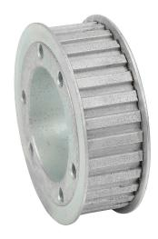
SureMotion timing pulley, ductile iron, 3/8in L pitch, 30 tooth, 3.581in pitch diameter, no hub with flanges. For use with 1in wide belt. Requires SDS series QD style bushing.
