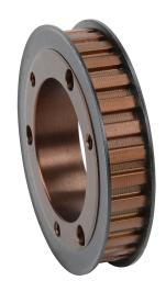
SureMotion timing pulley, ductile iron, 3/8in L pitch, 30 tooth, 3.581in pitch diameter, no hub with flanges. For use with 1/2in wide belt. Requires SDS series QD style bushing.
