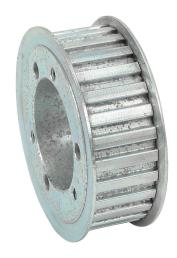
SureMotion timing pulley, ductile iron, 3/8in L pitch, 28 tooth, 3.342in pitch diameter, no hub with flanges. For use with 1in wide belt. Requires SH series QD style bushing.
