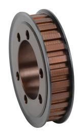
SureMotion timing pulley, ductile iron, 3/8in L pitch, 28 tooth, 3.342in pitch diameter, no hub with flanges. For use with 1/2in wide belt. Requires SH series QD style bushing.
