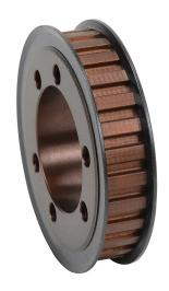
SureMotion timing pulley, ductile iron, 3/8in L pitch, 28 tooth, 3.342in pitch diameter, no hub with flanges. For use with 1/2in wide belt. Requires SH series QD style bushing.
