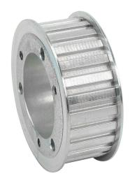
SureMotion timing pulley, steel, 3/8in L pitch, 26 tooth, 3.104in pitch diameter, no hub with flanges. For use with 1in wide belt. Requires SH series QD style bushing.
