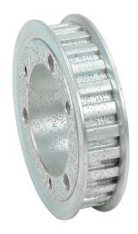
SureMotion timing pulley, steel, 3/8in L pitch, 26 tooth, 3.104in pitch diameter, no hub with flanges. For use with 1/2in wide belt. Requires SH series QD style bushing.
