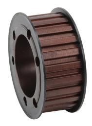
SureMotion timing pulley, steel, 3/8in L pitch, 24 tooth, 2.865in pitch diameter, no hub with flanges. For use with 1in wide belt. Requires SH series QD style bushing.
