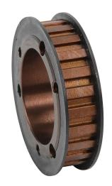
SureMotion timing pulley, steel, 3/8in L pitch, 24 tooth, 2.865in pitch diameter, no hub with flanges. For use with 1/2in wide belt. Requires SH series QD style bushing.
