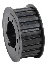
SureMotion timing pulley, steel, 3/8in L pitch, 22 tooth, 2.626in pitch diameter, no hub with flanges. For use with 1in wide belt. Requires JA series QD style bushing.
