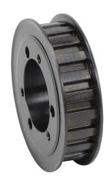
SureMotion timing pulley, steel, 3/8in L pitch, 22 tooth, 2.626in pitch diameter, no hub with flanges. For use with 1/2in wide belt. Requires JA series QD style bushing.
