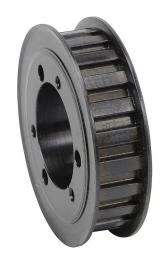
SureMotion timing pulley, steel, 3/8in L pitch, 22 tooth, 2.626in pitch diameter, no hub with flanges. For use with 1/2in wide belt. Requires JA series QD style bushing.
