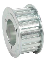
SureMotion timing pulley, steel, 3/8in L pitch, 20 tooth, 2.387in pitch diameter, no hub with flanges. For use with 1in wide belt. Requires JA series QD style bushing.
