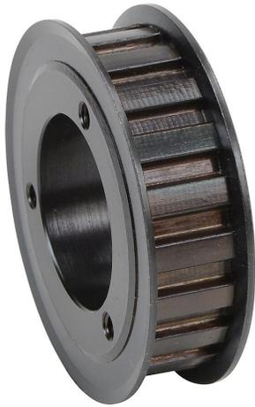
SureMotion timing pulley, steel, 3/8in L pitch, 20 tooth, 2.387in pitch diameter, no hub with flanges. For use with 1/2in wide belt. Requires JA series QD style bushing.
