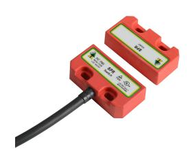
IDEM safety switch set, non-contact magnetic, (2) N.C. safety output(s), (1) N.O. monitoring output(s), plastic housing, 50 x 25mm, 8-pin M12 quick-disconnect, 9.8in/250mm cable length.
