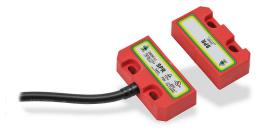
IDEM safety switch set, non-contact magnetic, (2) N.C. safety output(s), (1) N.O. monitoring output(s), plastic housing, 50 x 25mm, pigtail, 16.4ft/5m cable length.
