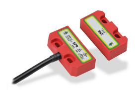
IDEM safety switch set, non-contact magnetic, (2) N.C. safety output(s), (1) N.O. monitoring output(s), plastic housing,  $50 \times 25$ mm, pigtail, 6.5ft/2m cable length.
