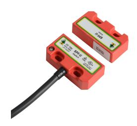
IDEM safety switch set, non-contact uniquely coded RFID, (2) N.C. safety output(s), (1) N.O. monitoring output(s), plastic housing, 50 x 25mm, 8-pin M12 quick-disconnect, 9.8in/250mm cable length.
