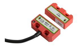
IDEM safety switch set, non-contact uniquely coded RFID, (2) N.C. safety output(s), (1) N.O. monitoring output(s), plastic housing, 50 x 25mm, pigtail, 32.8ft/10m cable length.
