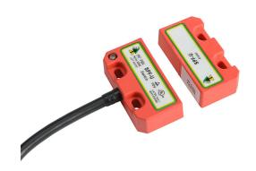
IDEM safety switch set, non-contact uniquely coded RFID, (2) N.C. safety output(s), (1) N.O. monitoring output(s), plastic housing,  $50 \times 25$ mm, pigtail, 16.4ft/5m cable length.
