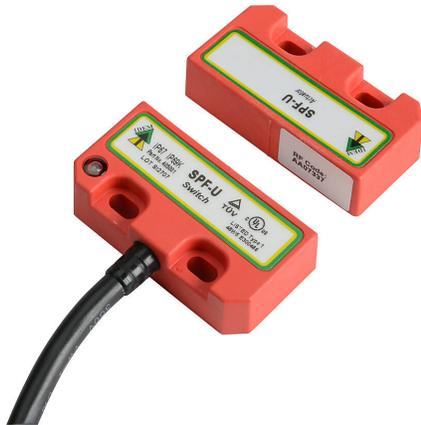
IDEM safety switch set, non-contact uniquely coded RFID, (2) N.C. safety output(s), (1) N.O. monitoring output(s), plastic housing, 50 x 25mm, pigtail, 6.5ft/2m cable length.
