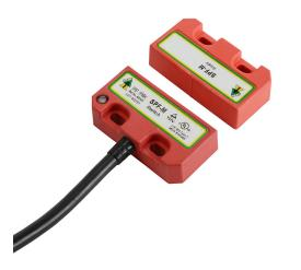
IDEM safety switch set, non-contact master coded RFID, (2) N.C. safety output(s), (1) N.O. monitoring output(s), plastic housing, 50 x 25mm, pigtail, 32.8ft/10m cable length.
