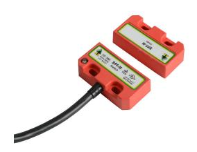
IDEM safety switch set, non-contact master coded RFID, (2) N.C. safety output(s), (1) N.O. monitoring output(s), plastic housing,  $50 \times 25$ mm, pigtail, 16.4ft/5m cable length.
