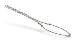
Bryant standard duty support grip, accepts cable diameter size 0.75 to 0.99in, closed, tin-coated bronze mesh, 13in length, single, eye length 8in, indoor and outdoor applications.
