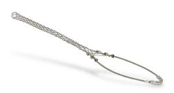
Bryant standard duty support grip, accepts cable diameter size 0.75 to 0.99in, closed, tin-coated bronze mesh, 13in length, single, eye length 8in, indoor and outdoor applications.
