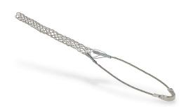
Bryant standard duty support grip, accepts cable diameter size 0.62 to 0.74in, closed, tin-coated bronze mesh, 10in length, single, eye length 8in, indoor and outdoor applications.
