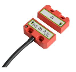
IDEM safety switch set, non-contact coded magnetic, (2) N.C. safety output(s), (1) N.O. monitoring output(s), plastic housing, 50 x 25mm, 8-pin M12 quick-disconnect, 9.8in/250mm cable length.
