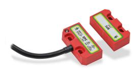
IDEM safety switch set, non-contact coded magnetic, (2) N.C. safety output(s), (1) N.O. monitoring output(s), plastic housing, 50 x 25mm, pigtail, 32.8ft/10m cable length.
